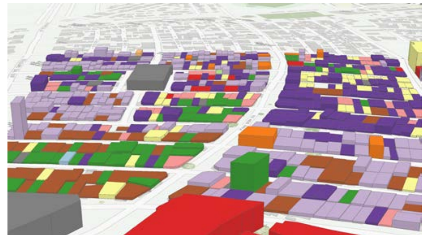
Figure 47: GIS representation, by colour and vertical extent, of the property values for individual land parcels in Dakar
